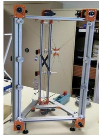
Fig. 2. Haptic interface device
