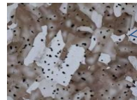
MIM-Ti grade 4 Structure monphasée alpha
