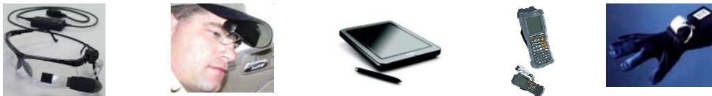
Figure 4: Goggles with integrated screen, See-Through goggles, TabletPC, RFID reader and Data glove
