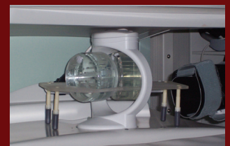
Figure 8: The phantom model simulating tibia at 30° of flexion in the MRI coil.
