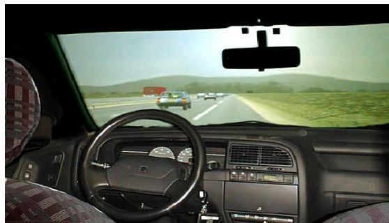
Figure 1. INRETS Driving simulator and visual environment simulated with ARCHISIM
